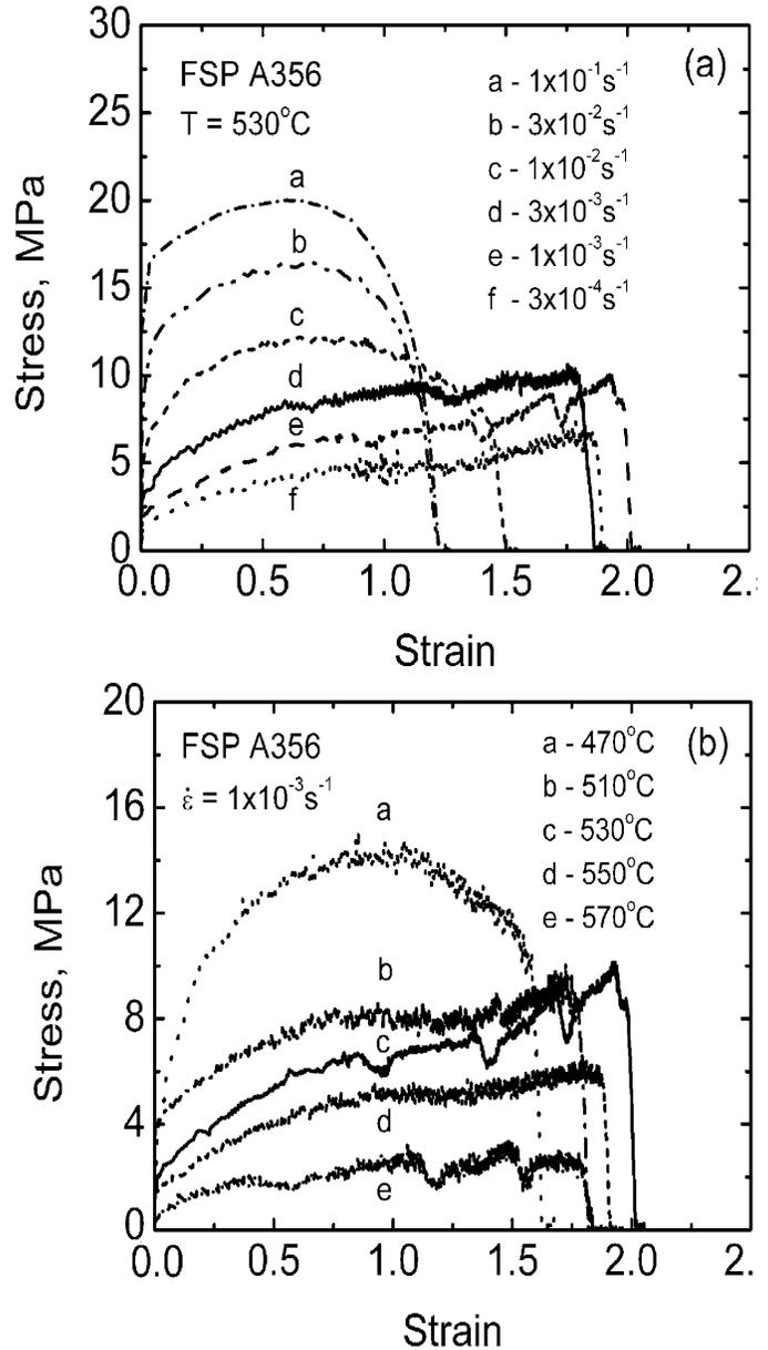
Figure 11: Stress–strain behavior of FSP A356 as a function of (a) initial strain rate at 530°C and (b) temperature at an initial strain rate of  $1 \times 10^{-3} \text{S}^{-1}$  [34]
