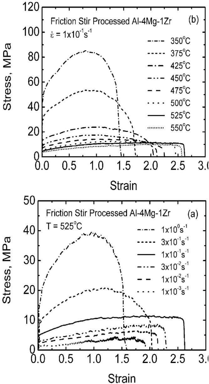
Figure 10: Stress strain behavior of friction stir processing Al-4Mg-1Zr, (a) initial strain rate at 525°C, (b) temperature at an initial strain rate  $1 \times 10^{-1} \text{s}^{-1}$  [33]
