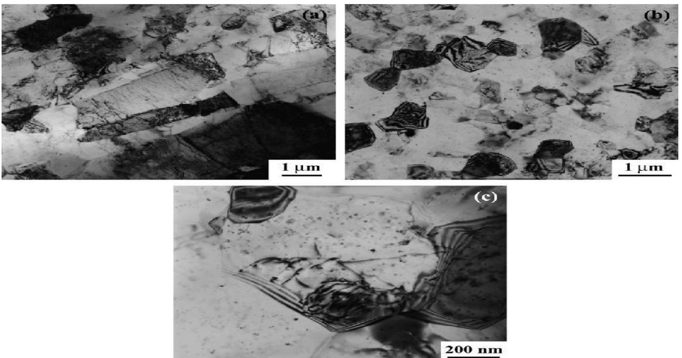
Figure 4: TEM images showing grain structure and dispersoid distribution in (a) as-extruded Al-Mg-Zr, (b) & (c) FSP Al-Mg-Zr [7]
