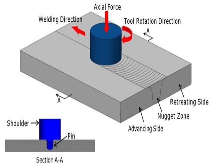
Figure 1: Friction Stir welding
